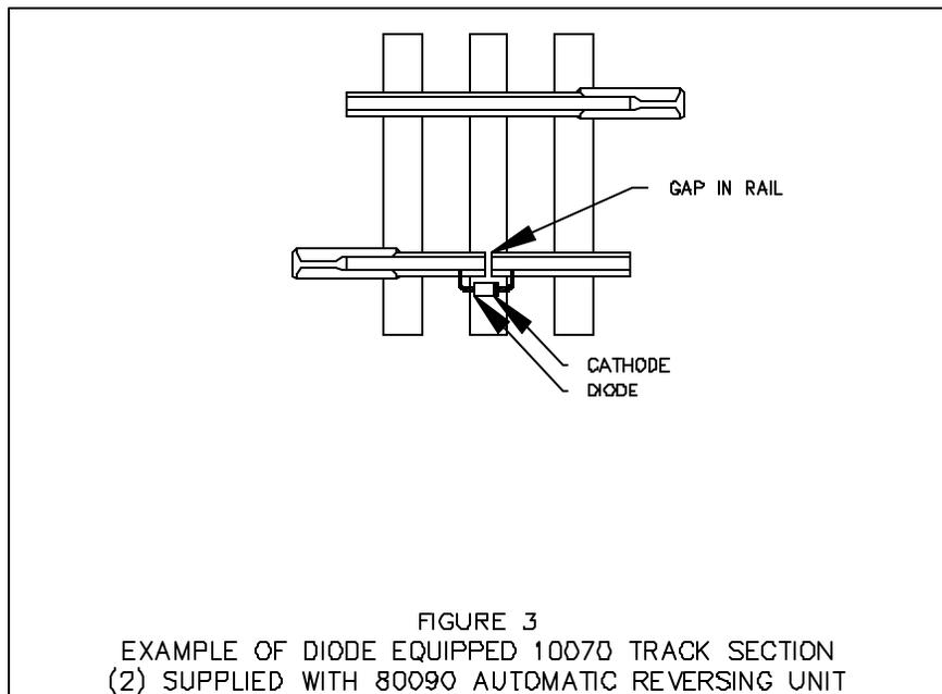
Simply take a LGB 10153 (old #1015U) track section, in which one rail is continuous and the other rail is split, remove its cover, and add a 1N5401 diode as shown in figure 4.
