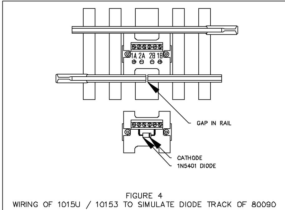
As an alternative, a LGB 10152 (old #1015T) section of track, which contains 2 split rails can also be used, by adding a wire jumper and 1N5401 diode as shown in figure 5.
